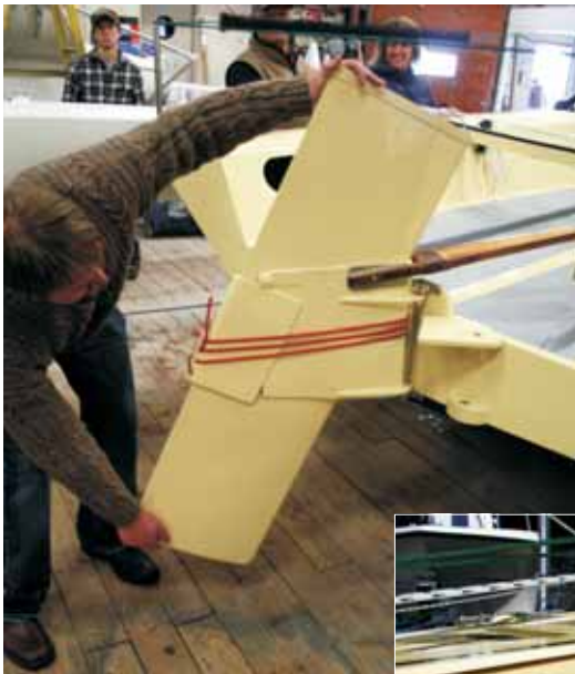
Left —Ben Gougeon demonstrates the blow-out safety feature of the rudder with a moveable trailing edge tensioned with shock cord.
