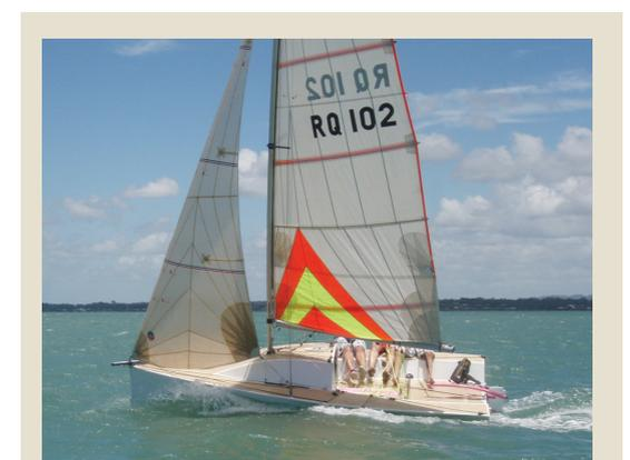
LOA 18'; LWL 17'6"; Beam 8'6" (overall), 4'7" (at waterline); Draft 5'; Displacement 800 lbs.; Ballast 180 lbs.; Sail area 236 sq. ft.; SA/D 43.82; D/L 66.63; L/BWL 3.93
