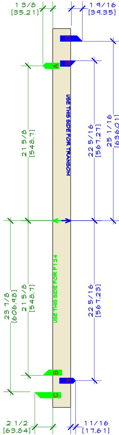
Hull bottom measurement jig,
