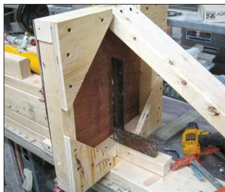
**Above**—When CCI partners Dave Brady and Phil Locker decided to build an 18' (5.5m) i550 sportboat designed for construction in 1/4" (6mm) plywood, they tested composite panels as possible substitutes. **Above right**—The hand-pumped hydraulic ram pushes on the gelcoat side of a panel. **Right**—The first test employed a square on the back side of the panel to measure the potential oilcanning of the hull.
